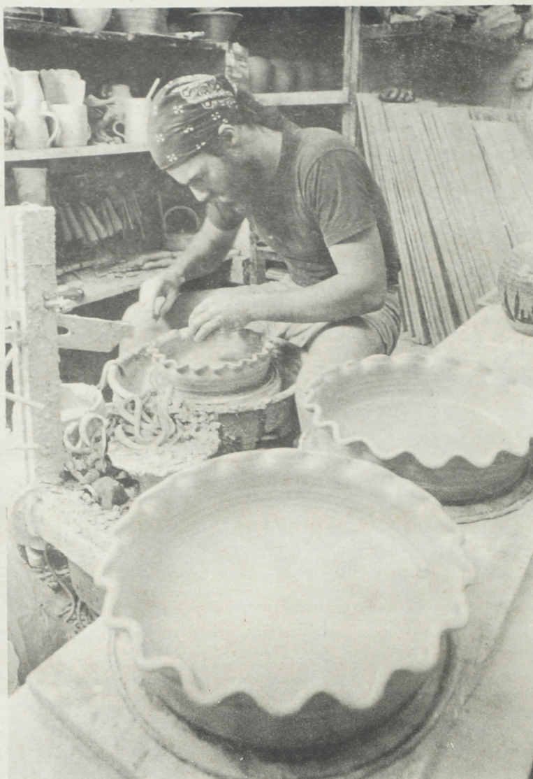
WHERE IT ALL BEGINS is the wheel on which most of the pots are shaped (some pieces are done by extrusion or are rolled). David Hevener is at work on several quiche baking dishes here.
