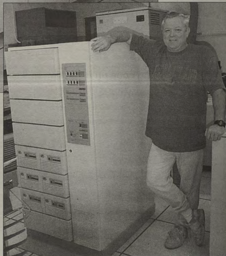
NEWER TECHNOLOGY — FIVE GB IN EACH OF THESE 'DRAWERS': Russ next to a stack of IBM "RAMAC" drives, manufactured during the last five years. Each horizontal "drawer" holds five gigabytes of memory.
