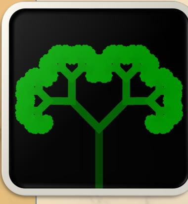
fractal get shorter with each recursion. Drawing stops when a threshold length is reached.
