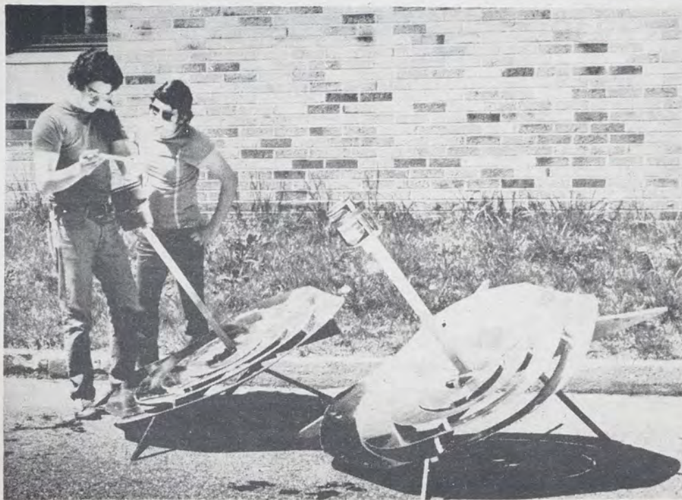
Mark Vendettuoli and Leo Larivee demonstrate the solar cookers they designed and built for their Industrial Arts course. The course, "Power Systems Development," or I.A. 222, provided the students with the opportunity to experiment with solar energy. The cookers are capable of boiling water without any energy other than the sun. Anchor Photo/Bruce Sumner.
